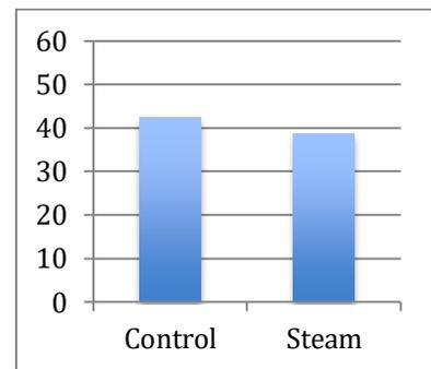
When exposed to autoclave conditions, MPU 100 demonstrates a 6% increase in elongation at break, a 18% drop in modulus and a 9% drop in ultimate strength. **Despite these small changes in mechanical properties, parts readily deformed immediately after autoclave and remained soft for several hours afterwards. Carbon does not recommend high temperature sterilization for MPU 100.**
